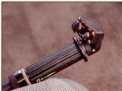
A throttle governor correlates collective and power. Three 330s (left to right): three seats, two controls; three and three; and the four-person luxu version.
